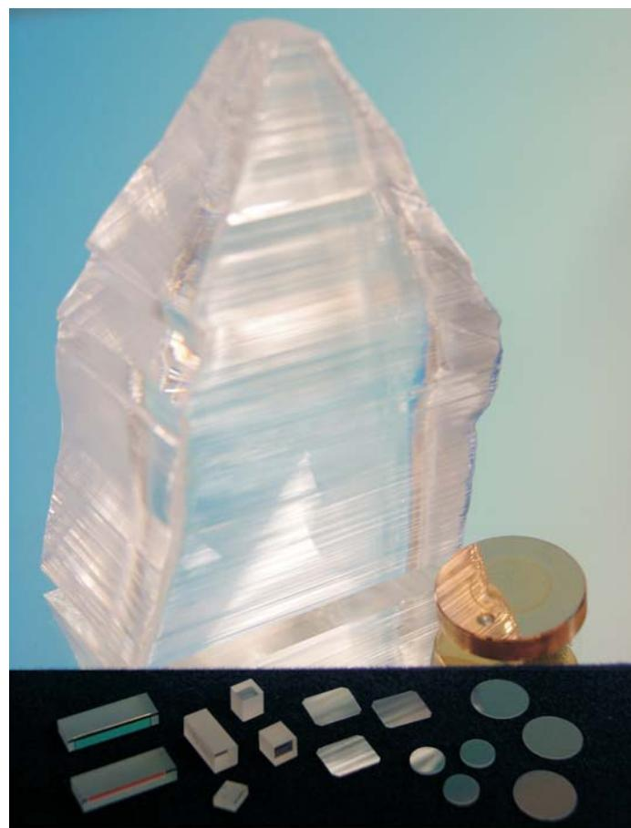
**Yb<sup>3+</sup> doped KGW and KYW single crystals are known as the best laser active material for diode or laser pumped solid-state laser. VCT AG is now presenting Yb<sup>3+</sup> doped KLW, with the possibility of Yb doping higher than 16at.%. Basic optical and laser properties are expected to be like Yb<sup>3+</sup> doped KGW and KYW.**
