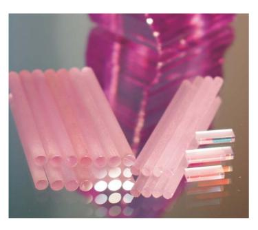
Nd<sup>3+</sup> doped KGW single crystals are known for their high efficiency (3-5 times higher than Nd:YAG lasers). VCT AG supplies not only high optical quality of the crystals, also guaranteed precise optical orientation. This is ensured by complex crystal qualification on a high scientific level, leading to reliable reproducibility.
