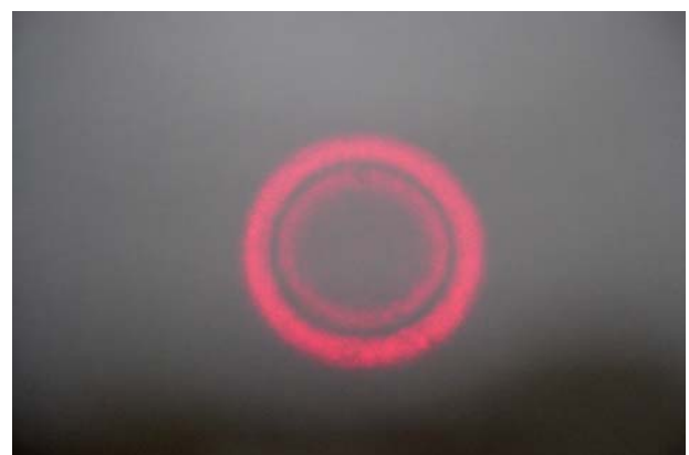
Fig. 7: Magnified and on screen projected light- and Poggendorff rings, resulting from internal conical refraction with a 20 mm long MDT- crystal of the VCT AG.
