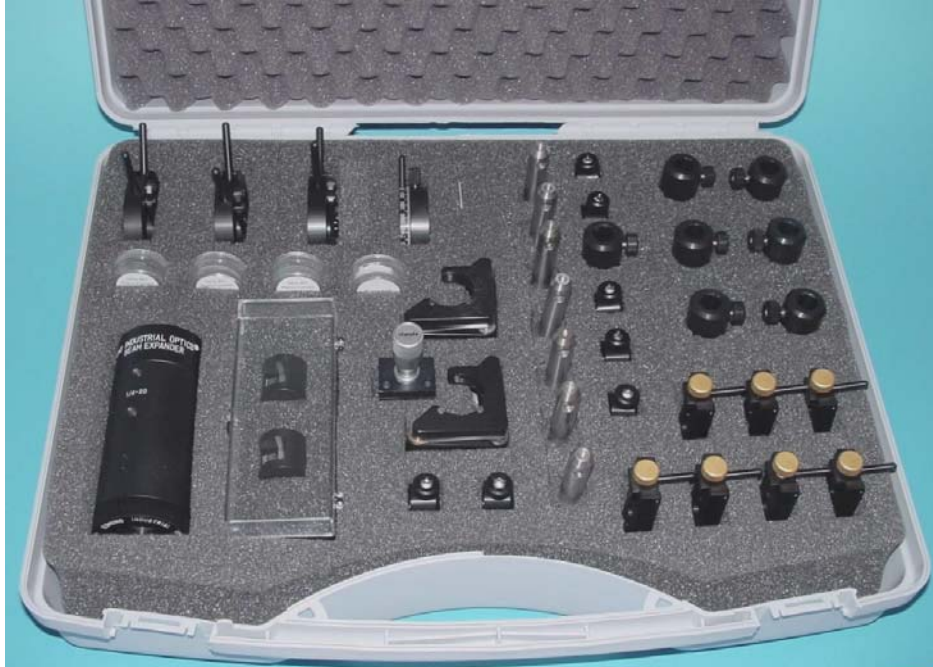
Fig. 1: Education kit of the VCT AG for internal and external conical refraction
